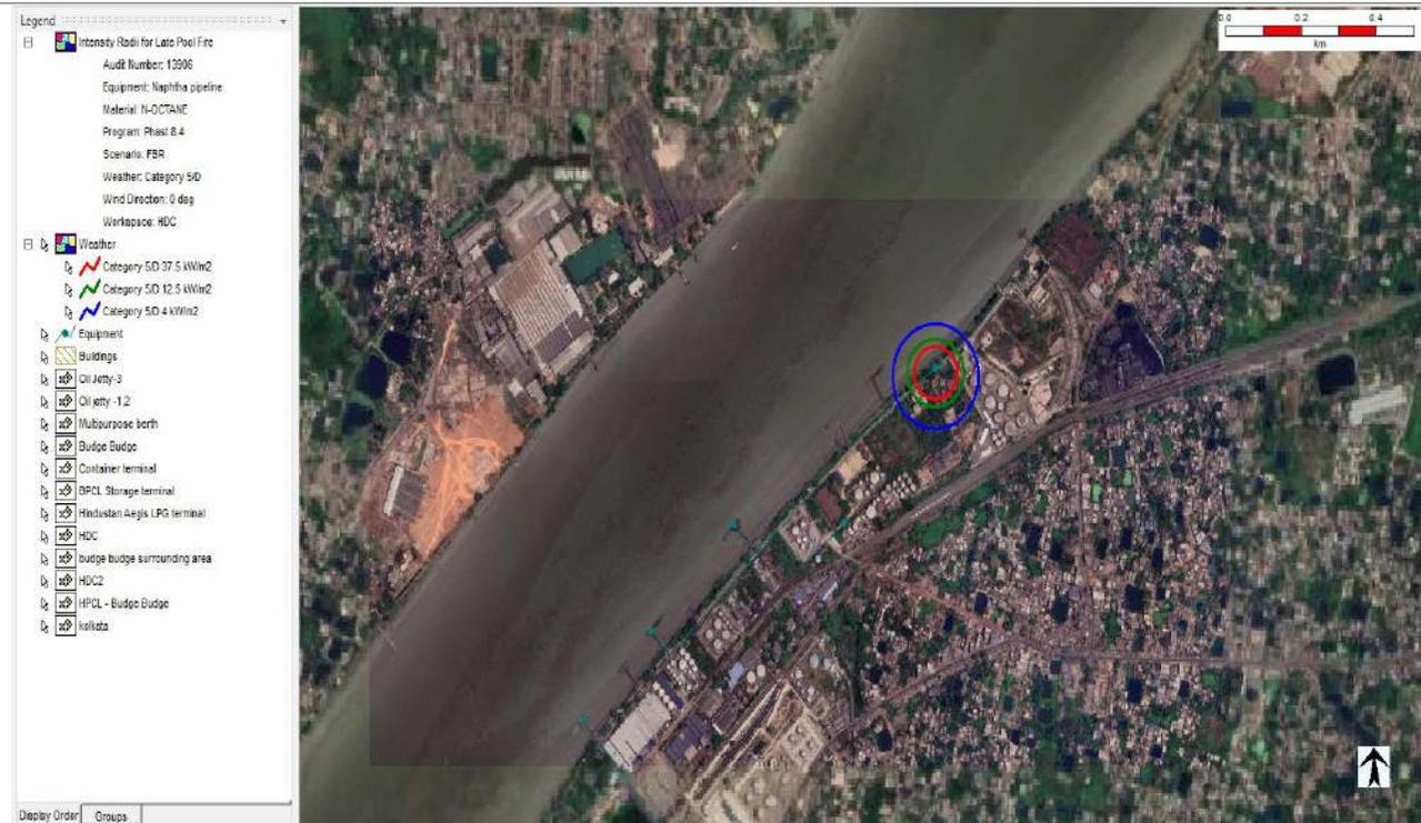
15. Pool fire from Full Bore Rupture of MS unloading hose with wind speed 5 m/s and D stability class at Budge Budge Oil Jetty-1.
