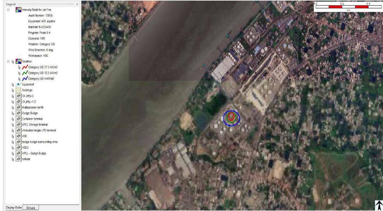
21. Pool Fire from Full Bore Rupture of ATF transfer pipeline with wind speed 5 m/s and D stability class from jetty to terminal.
