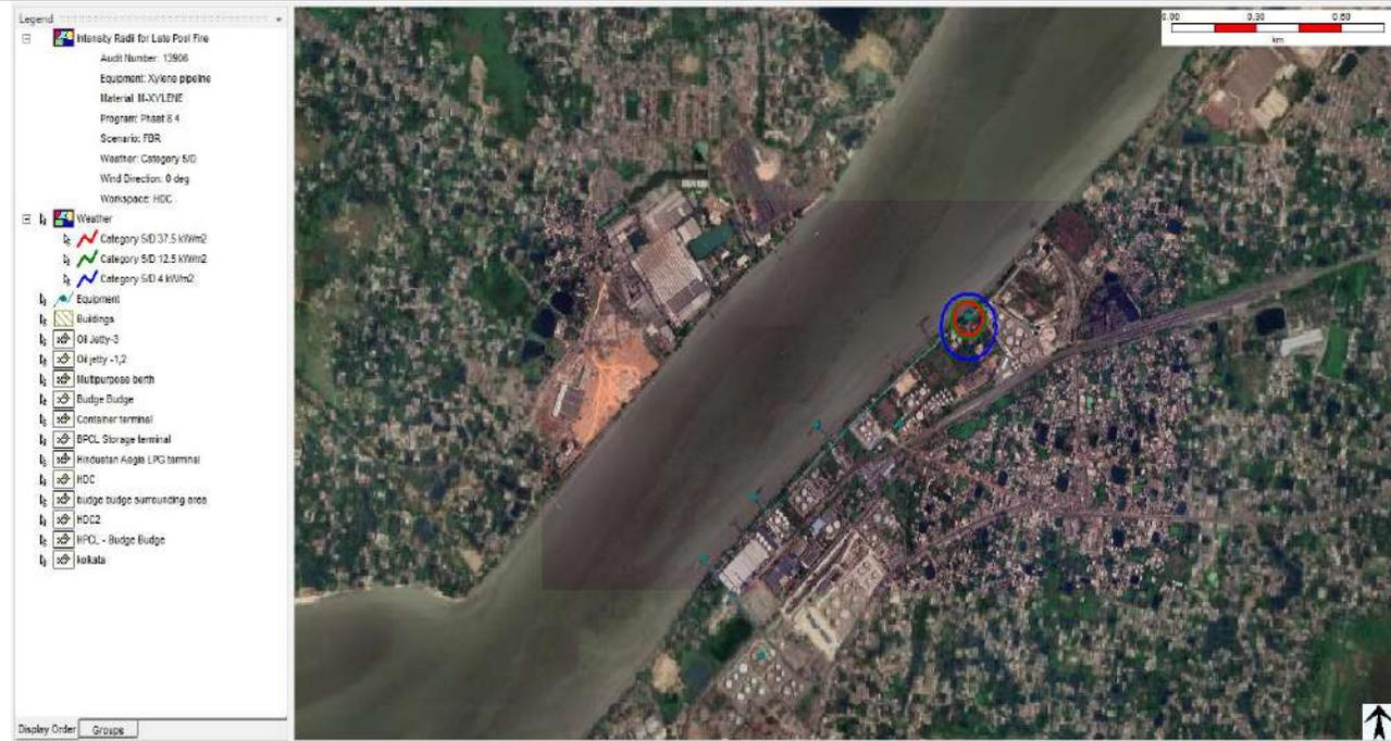
14. Pool fire from Full Bore Rupture of **Naphtha** transfer pipeline with wind speed 5 m/s and **D** stability class from jetty to terminal.
