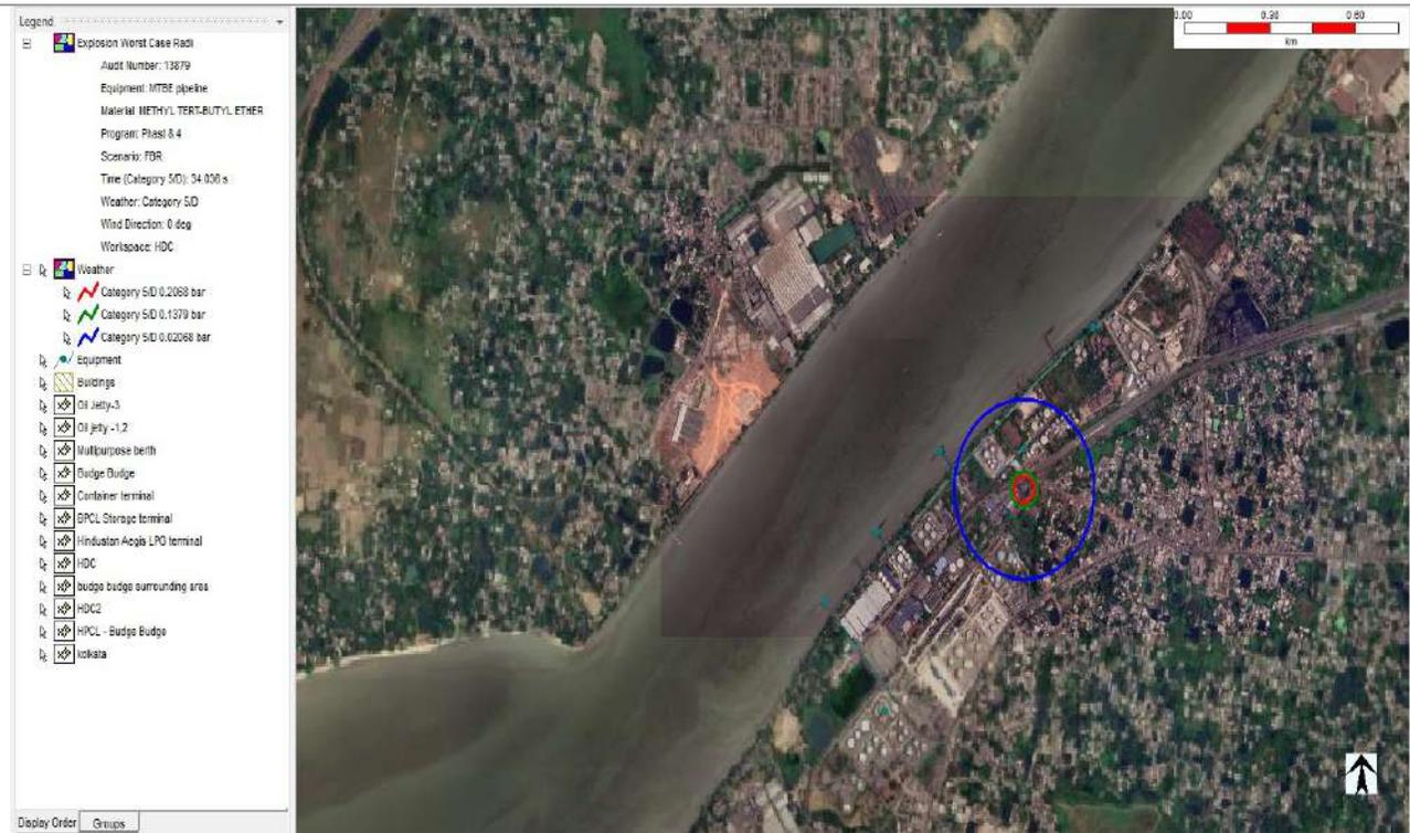
**8. Pool fire from Full Bore Rupture of Toluene unloading hose with wind speed 5 m/s and D stability class at Budge Budge Jetty-3.**
