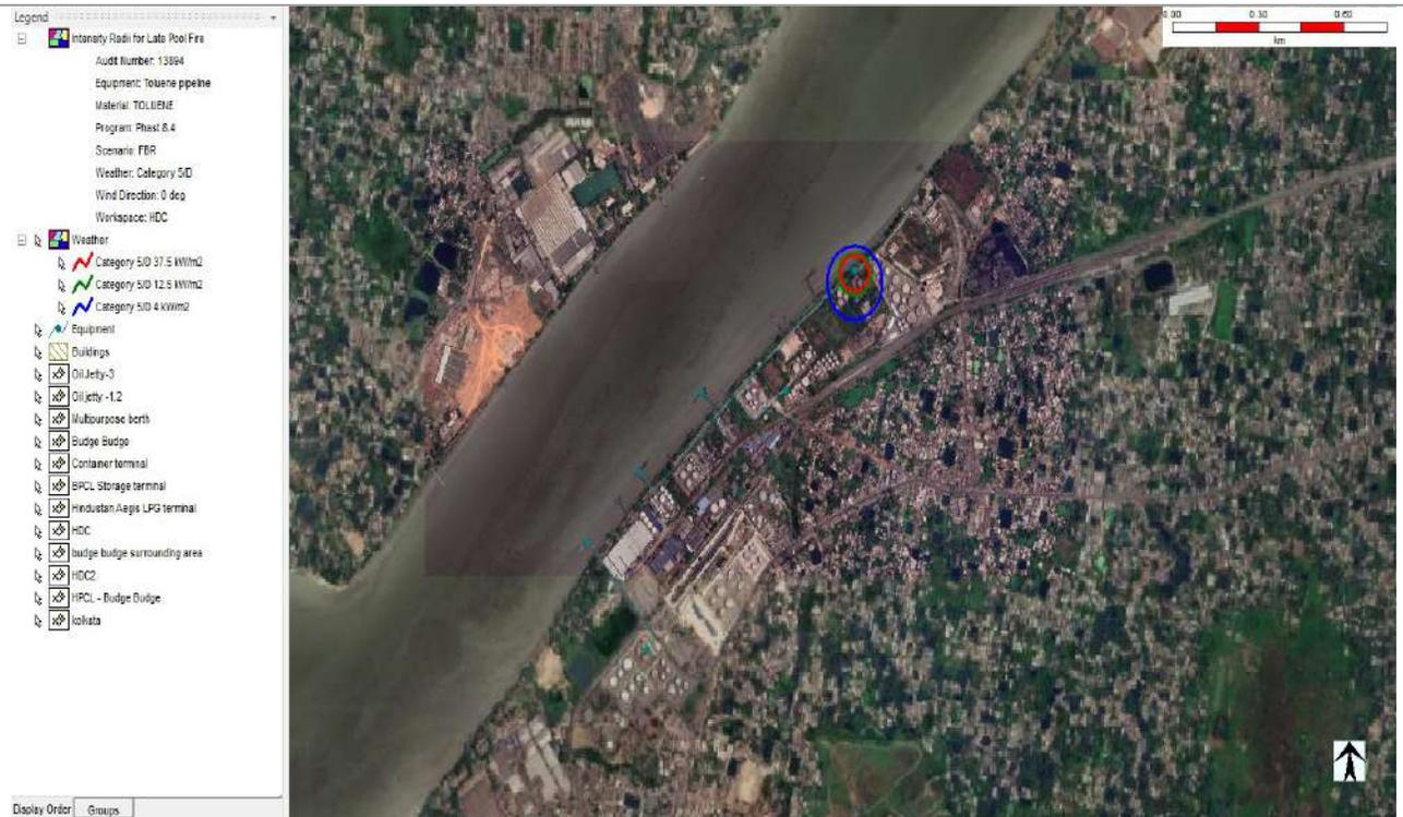
13. Pool fire from Full Bore Rupture of **Xylene** transfer pipeline with wind speed 5 m/s and **D** stability class from jetty to terminal.
