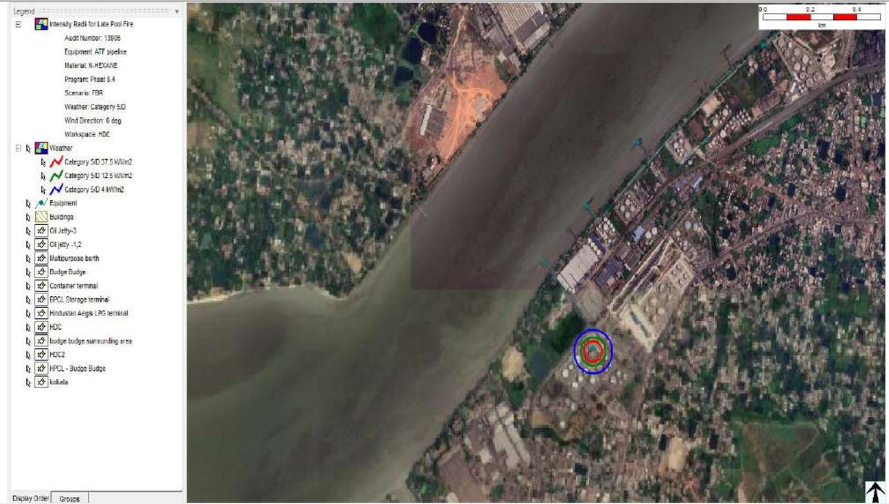
22. Vapor cloud explosion from Full Bore Rupture of ATF transfer pipeline with wind speed 5 m/s and D stability class from jetty to terminal.
