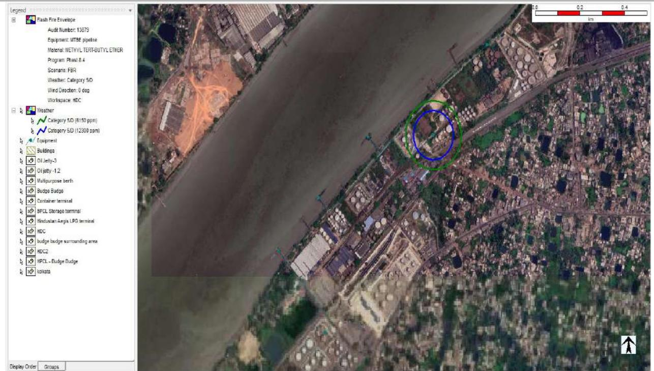
**7. Vapour cloud Explosion from Full Bore Rupture of MTBE transfer pipeline with wind speed 5 m/s and D stability class from jetty to terminal.**
