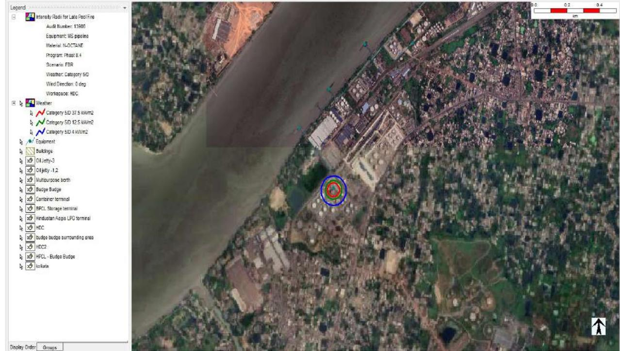
20. Jet Fire from Full Bore Rupture of ATF transfer pipeline with wind speed 5 m/s and D stability class from jetty to terminal.
