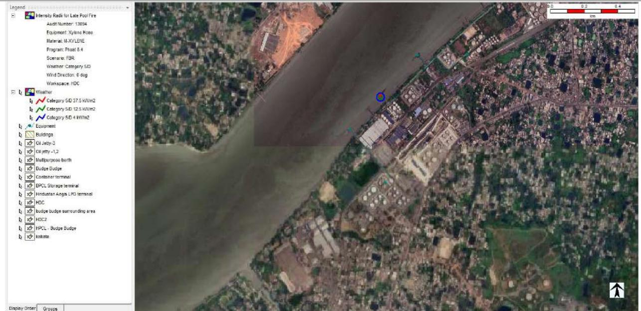
10. Jet fire from Full Bore Rupture of MS transfer pipeline with wind speed 5 m/s and D stability class from jetty to terminal.
