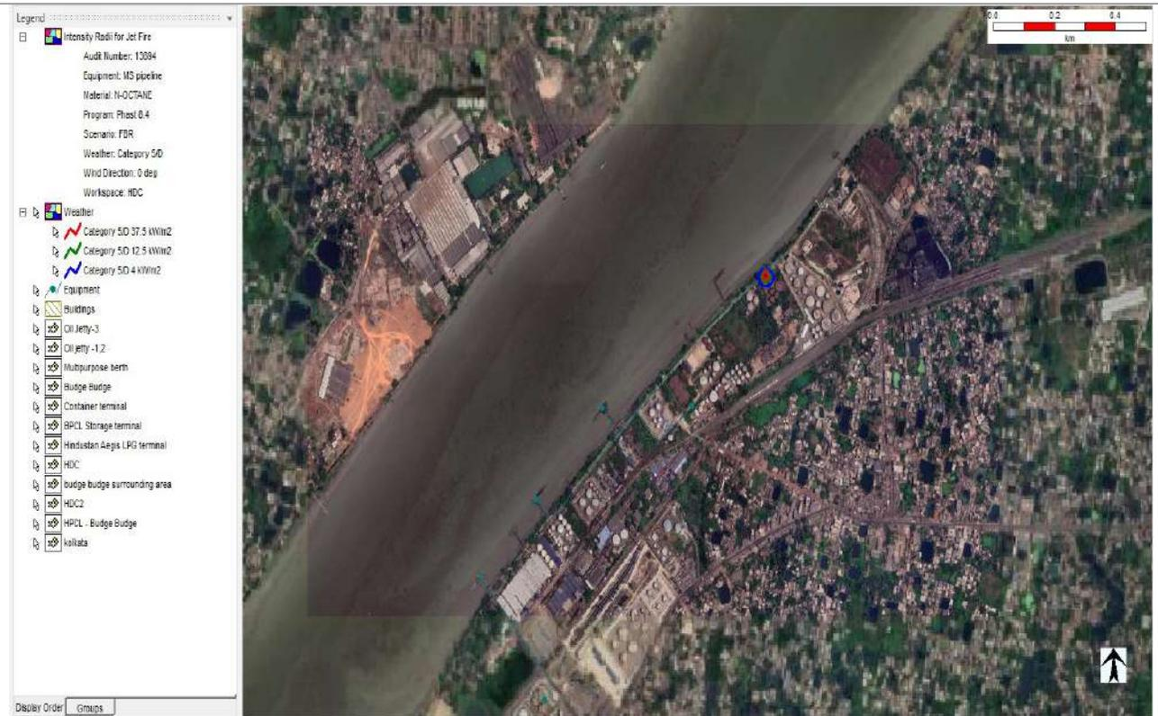
11. Pool fire from Full Bore Rupture of MS transfer pipeline with wind speed 5 m/s and D stability class from jetty to terminal.
