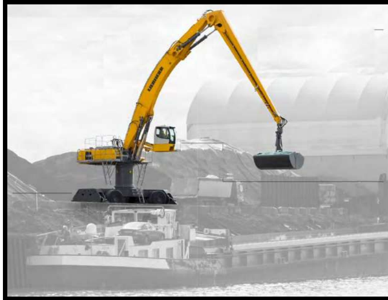
TYPICAL BARGE UNLOADER FOR BARGES
