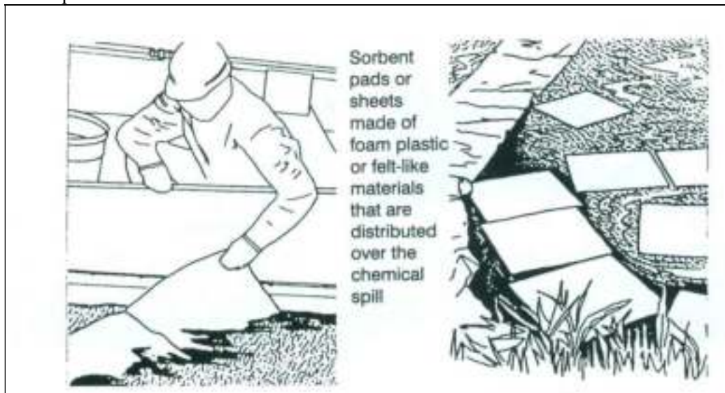
Figure I.2: Treating a HNS spill on the water surface with sorbent plates or pads
