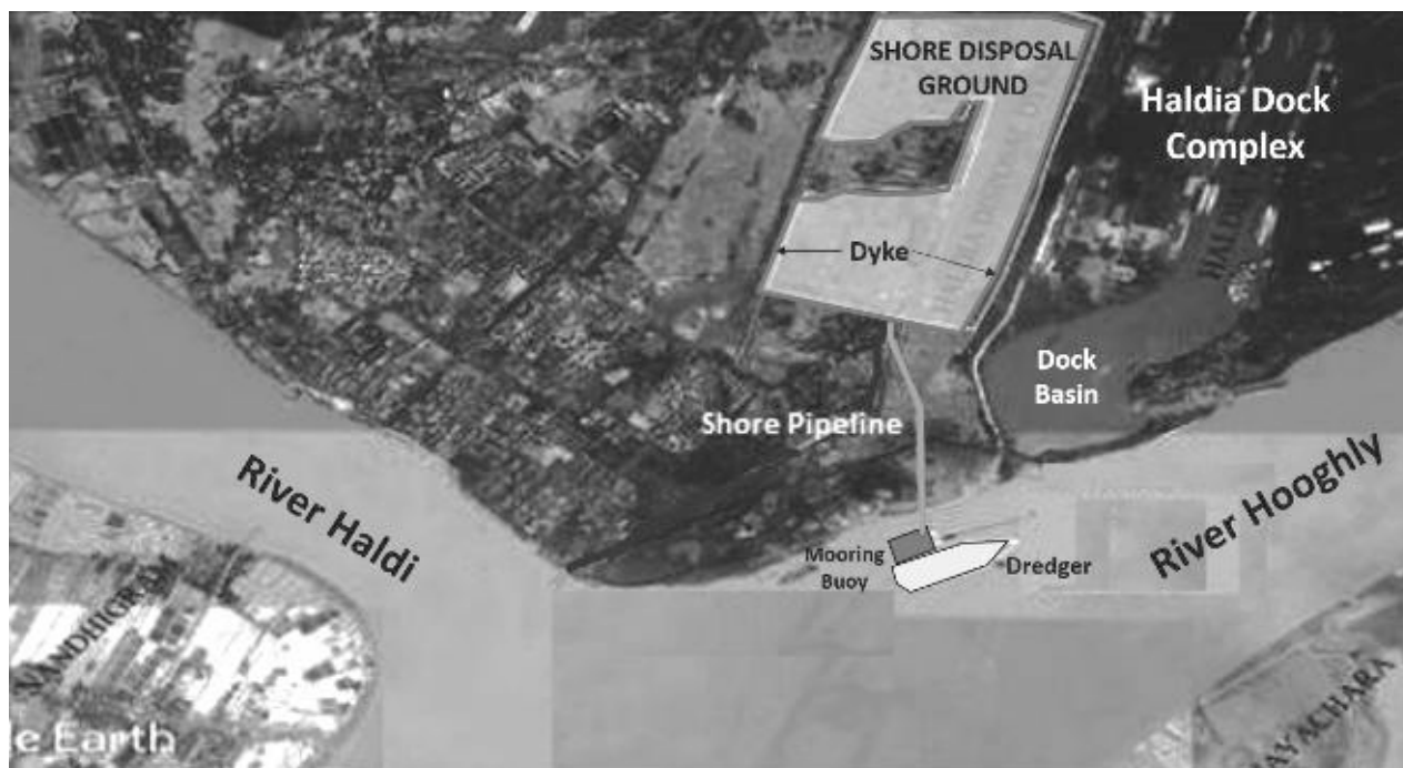
Proposed Dyke at Haldia for Shore Disposal
