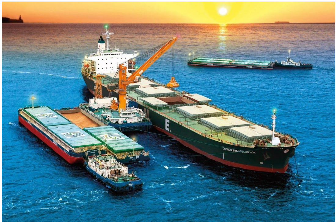
Figure Q: Cargo handling by Floating Crane
