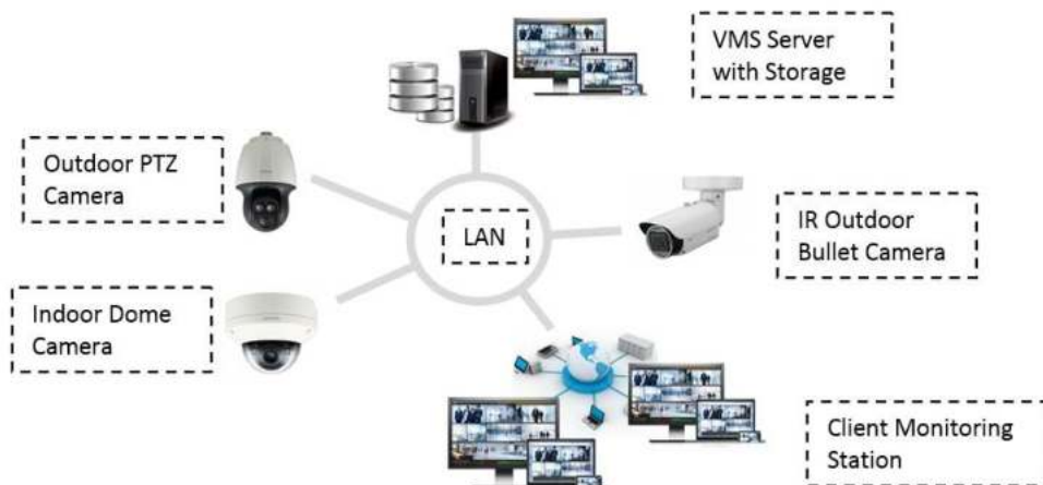
Figure 63 Conceptual Schematic of IP Based CCTV System
