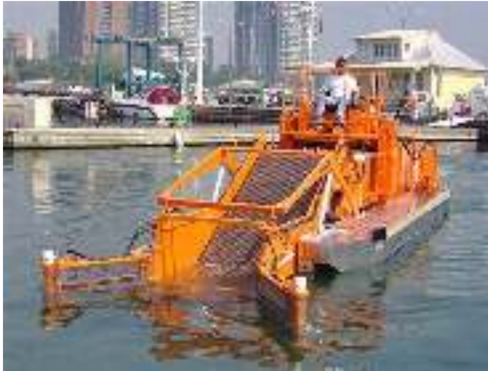
Figure 12 Typical Debris Removal Boat
