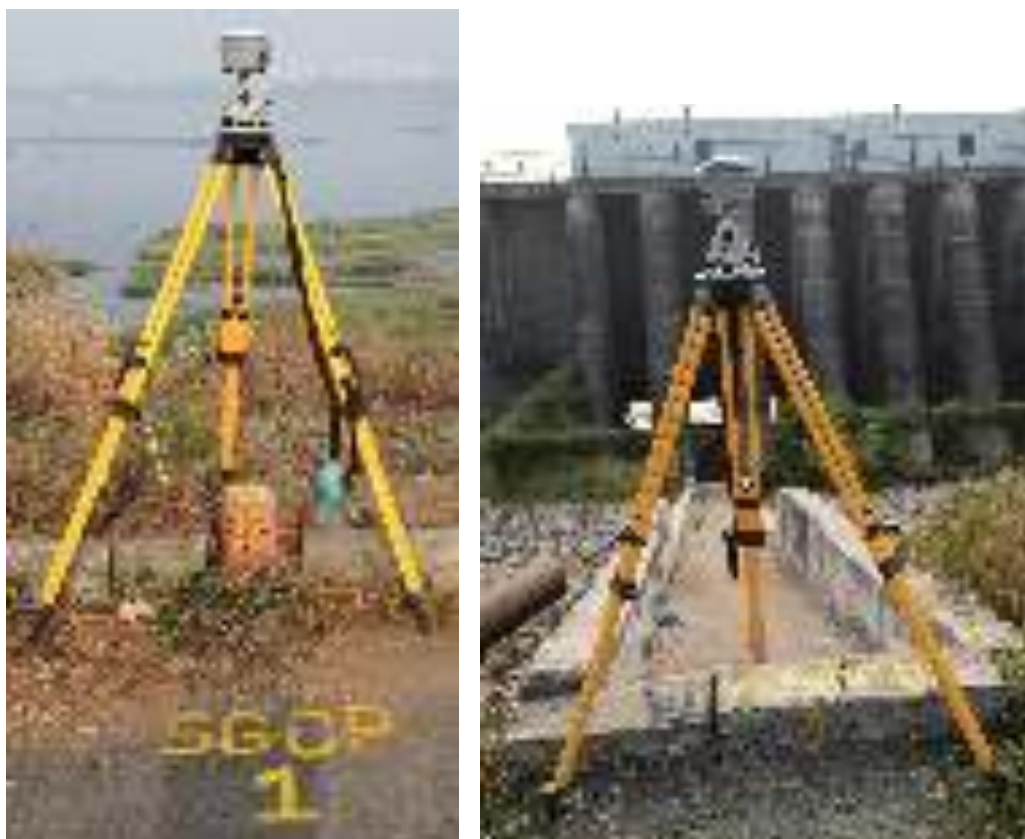
FIGURE 29 ESTABLISHMENT OF SECONDARY GROUND CONTROL POINT
