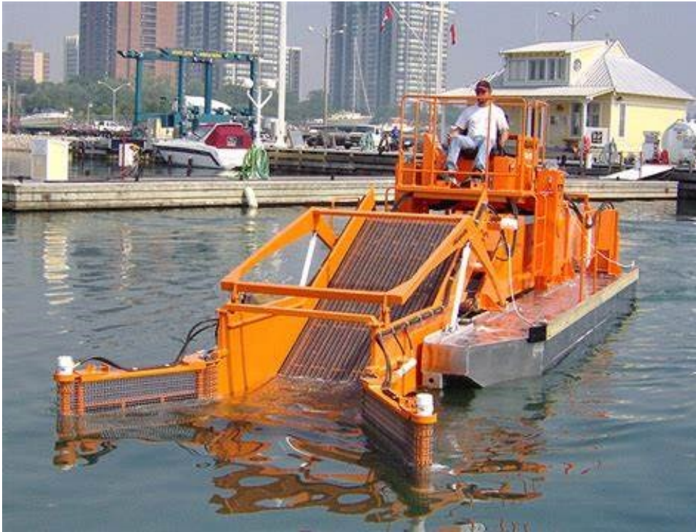
Figure 11 Typical Debris Removal Boat
