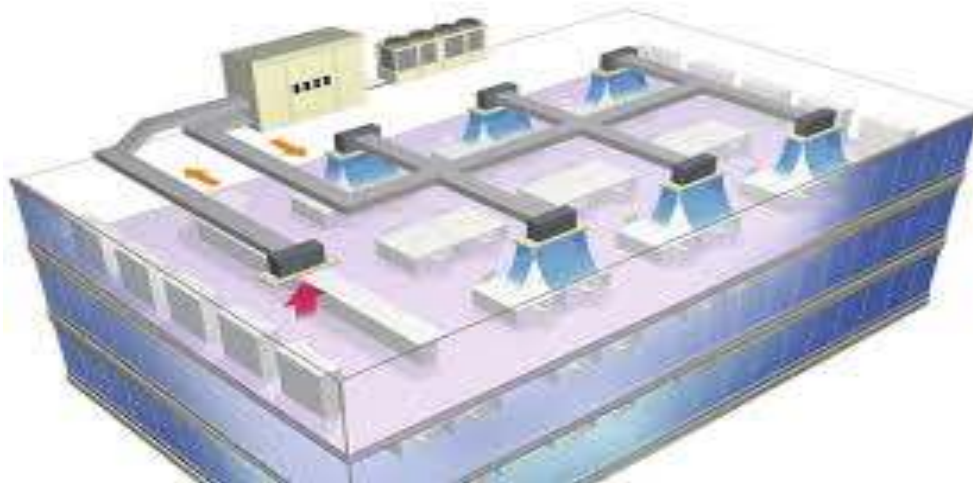
FIGURE 80 VRV SYSTEM ILLUSTRATIVE LAYOUT
