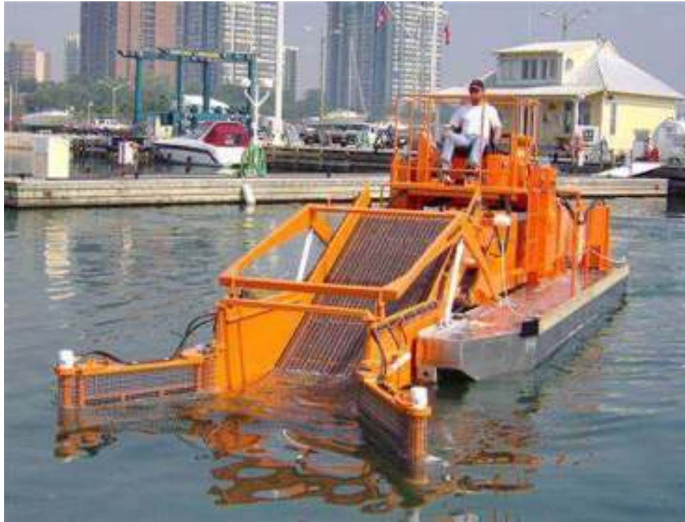
Figure 12 Typical Debris Removal Boat
