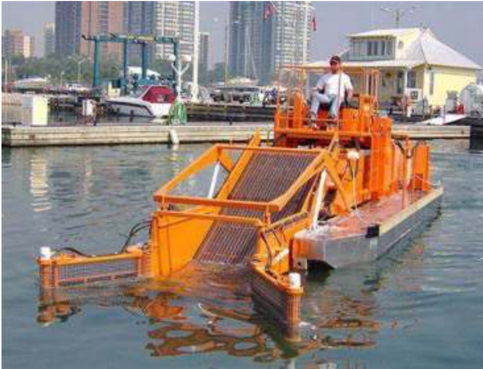
Figure 11 Typical Debris Removal Boat
