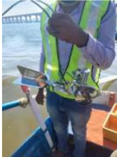
FIGURE 35 CURRENT VELOCITY AND DISCHARGE MEASUREMENT INSTRUMENT
