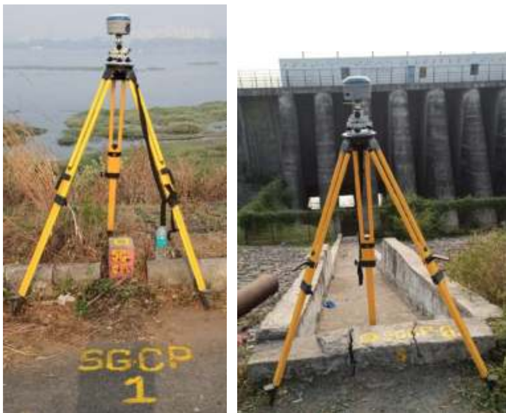
FIGURE 29 ESTABLISHMENT OF SECONDARY GROUND CONTROL POINT
