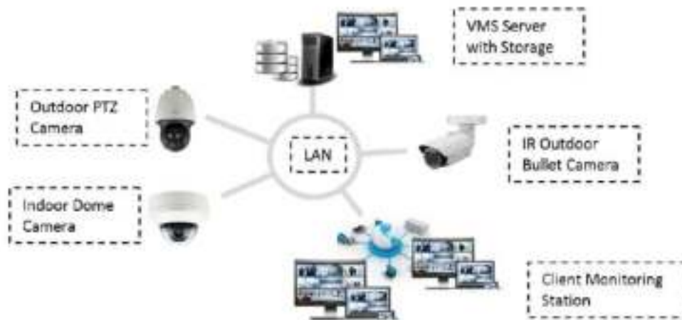
Figure 63 Conceptual Schematic of IP Based CCTV System
