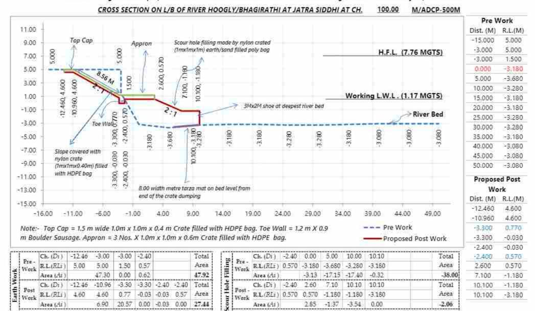
Note:- \* Length of Slope for Pitching = 8.56 M . \*\*Area in Sam. Ai = 0.50 x [D(i+1) - Di] x [RLi + RL(i+1)]
