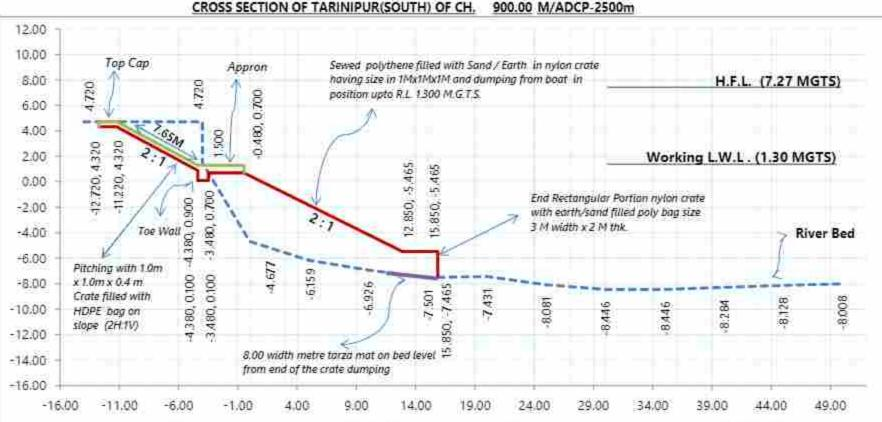
Note: Top Cap = 1.5 m wide 1.0m x 1.0m x 0.4 m Crate filled with HDPE bag. Toe Wall = 1.2 m X 0.9 m Boulder Sausage. Appron = 3 Nos. X 1.0m x 1.0m x 0.6m Crate filled with HDPE bag.
